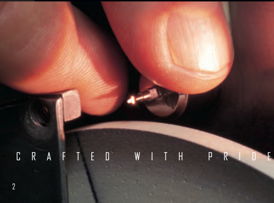
(Below) Precision grinding of the tiny orifice cutting tools used on Hago's production lines is also done in-house to maintain total quality control, from start to finish.
