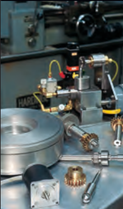
(Left) A sampling of the exotic machine components, pneumatic controls and stepping motors used in the construction of Hago's highly automated production machinery.
